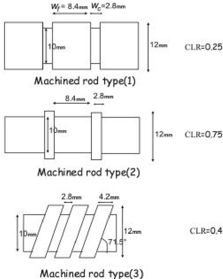
$$\text{Concrete Lugs Ratio (CLR)} = \frac{\text{concrete width}}{\text{(concrete + CFRP) width}} = \frac{W_c}{W_c + W_f}$$
